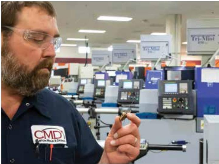
Swiss turning can quickly and accurately make long, thin parts like this core pin, and make most parts in a single operation without custom fixturing.
