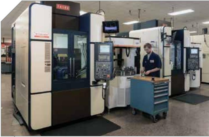
Yasca micromachining centers equipped with robotic part changers perform precision five-axis machining unattended in continuous operations through the weekend.
